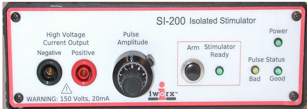
Figure HP-11-S1: The front panel of the SI-200 with the two high voltage (H.V.) output sockets, the amplitude control knob with its indicator dial, and the power and high voltage status lights.
