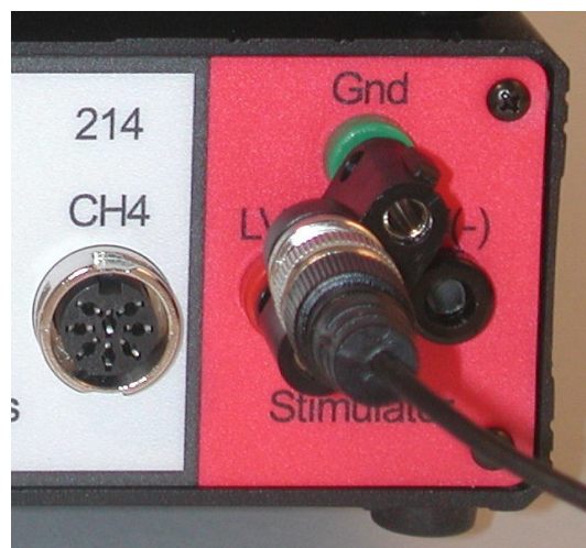
Figure HP-11-S5: The Female BNC to Dual Banana Adapter and BNC-BNC cable connected to the stimulator output of an IWX/214.
