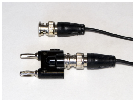
Figure HP-11-S4: BNC-BNC cable attached to a female BNC to Dual Banana adapter. The tab on the side of the adapter identifies the prong that is connected to the ground jack.
